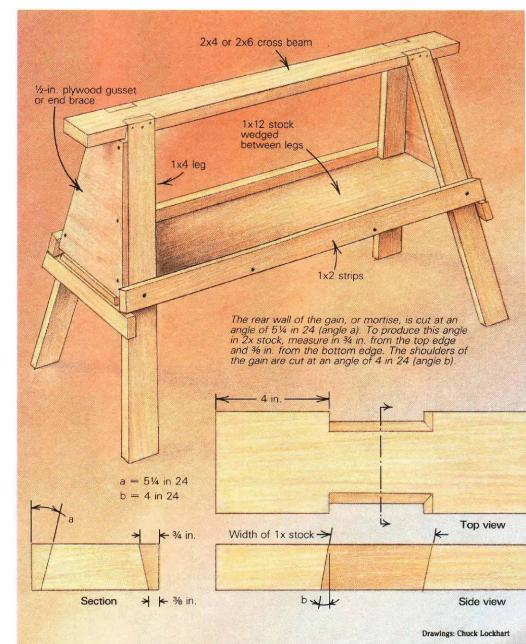
or 2x6 and cut it to a length of 42 in. The legs of a well-made trestle have to be let into the cross beam, so the next thing I do is lay out the four mortises, or gains, that will receive the tops of the legs. Because the legs splay in two directions, the shoulders of the gain slope in one direction and the rear wall of the gain in another (bottom drawing, facing page).
